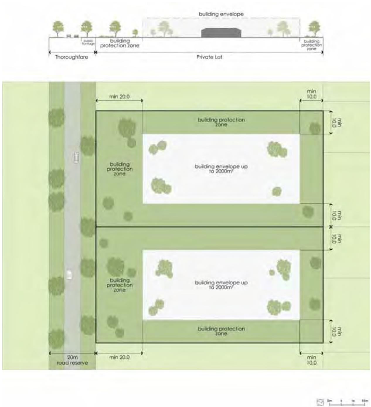
FIGURE 9 INDICATIVE BUILDING ENVELOPES AND CROSS-SECTION – TYPICAL LOTS
