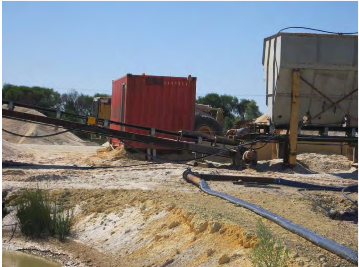
Figure 4 – The Feed Hoper (“F”) supplies the Trommel Feed Conveyor (Area “E”).
