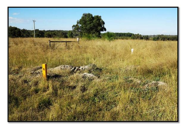
Figure 8 Typical part of Lot 7 showing the DSY water monitoring bore (white) and Main Roads water monitoring bore (yellow)
