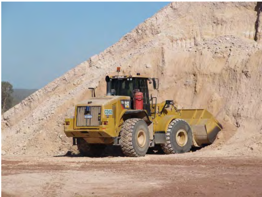
Recovering clay from stockpile
