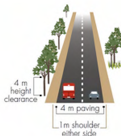
Figure 19: Minimum design requirements for a public road
