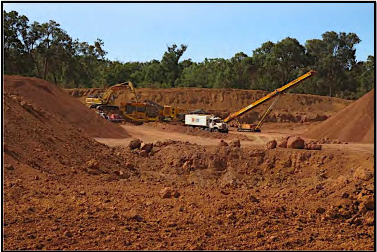
Figure 7: Crushing laterite duricrust on the pit floor to maximise noise and dust
