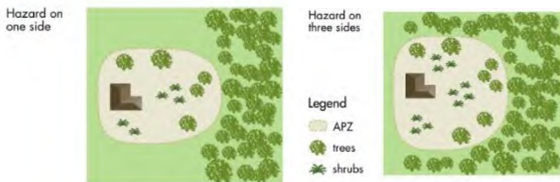
Figure 25: Design of an Asset Protection Zone
