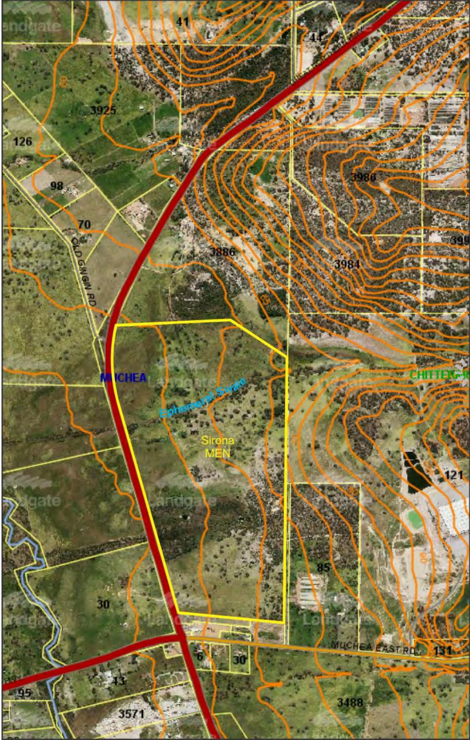
Figure 4 Contour map (5m contour lines) of the Harvis MEN development showing ephemeral swale
