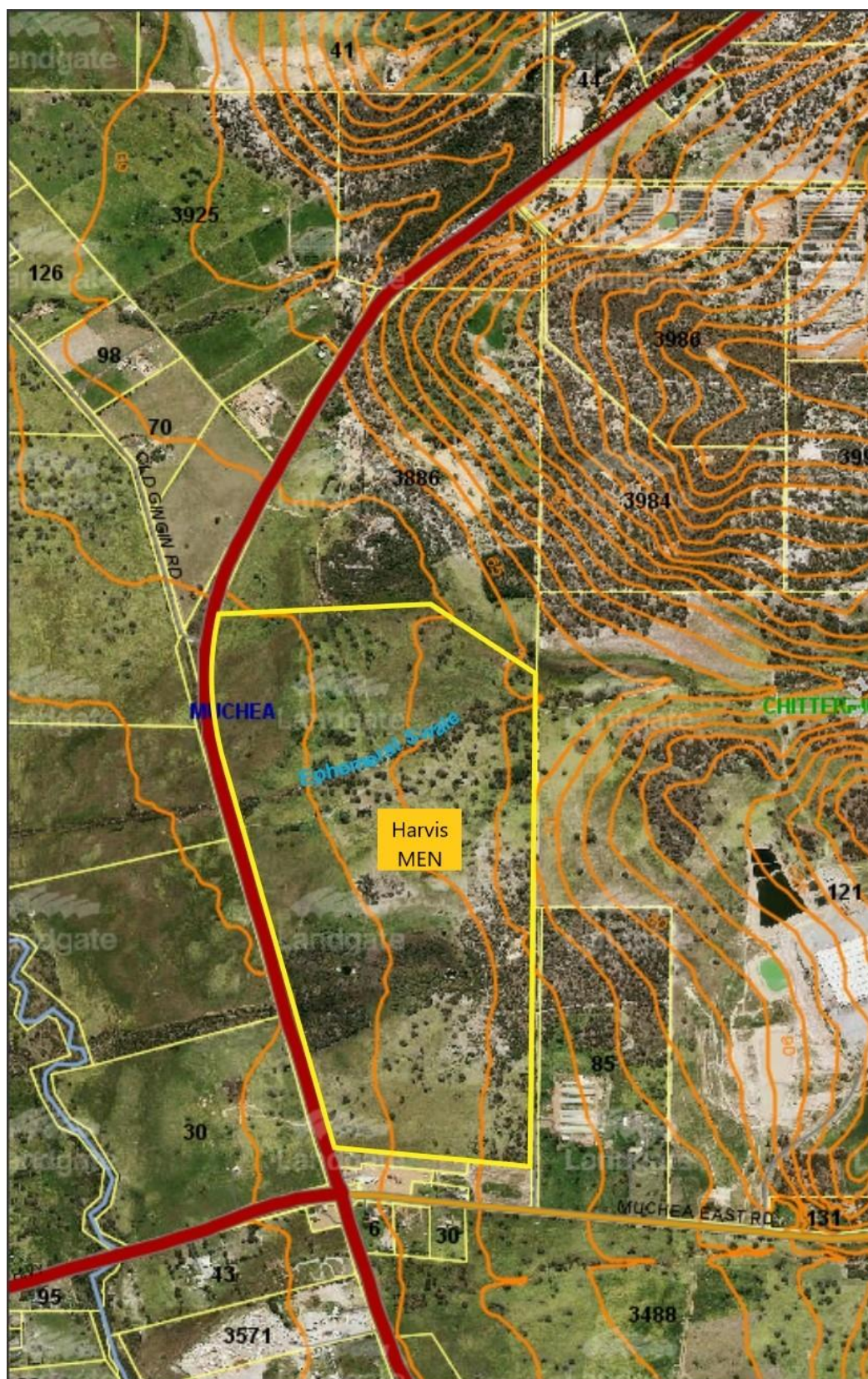
Figure 3: Contour map (5m contour lines) of the Harvis MEN development showing ephemeral swale
