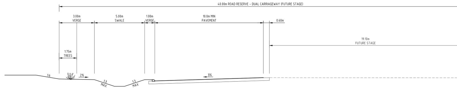
TYPICAL CROSS SECTION OF LOOP ROAD - STAGE 1
